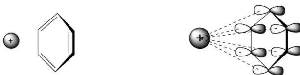
Fig.II.3.1 The interaction cation- \pi between a random cation and an aromatic benzene ring [adapted from UC Davis ChemWiki].
